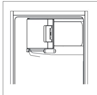
8. Unscrew bottom hinge. Then remove the adjustable feet from both side.
