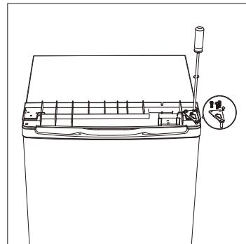
4. Unscrew bottom hinge of freezer door. Then remove the door and place it on a soft pad to avoid scratch.
